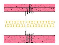
120/120 Minutes (Integrity/Insulation). BTC 17442F - BRE Report P102396-1011A **Refer to Speedline Specification Clause** 154 mm. (At Base Track, Excluding Finishes) Severe - Annexes A-F 50 R<sub>w</sub>dB, Date Tested or Assessed Against - 70-B-57(25)
